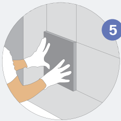
5 | ALIGN The rafts to the shapes and adhere to the underlying surface by applying pressure.
