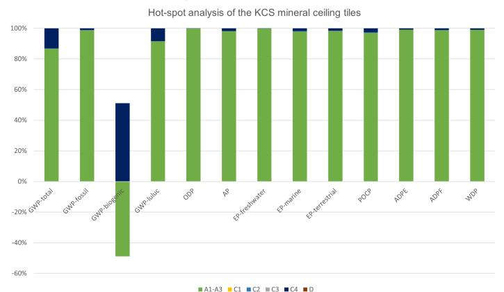
The comparison of the product's life cycle phases shows a clear dominance of the production phase (modules A1–A3) in all environmental impact categories. The potential environmental impacts from transport to disposal (module C2) and the End-of-Life of the products due to landfilling (module C4) have a minor contribution.
